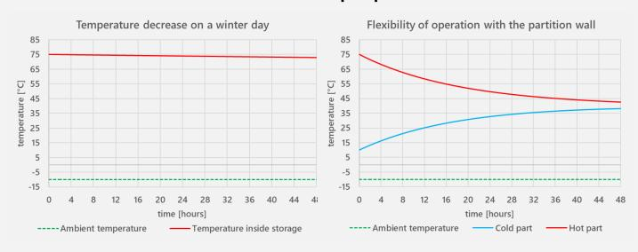
The heat inside the battery is not lost but only transferred from the hotter to the colder part – it is cheaper to heat up the water to the desired temperature and also, the battery maintains high flexibility of operation.
